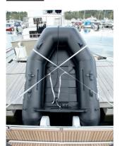
Always fasten the dinghy with two crossed ropes to the boat (not included), as wide as possible, for stability. Use the D-rings designed for towing, on the dinghy tubes.
